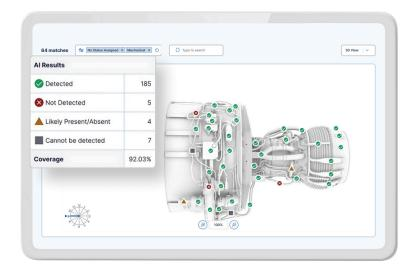
The system detects and verifies engine components in near real-time using high-resolution images captured via robotic or handheld devices. Al-powered models analyse the captured data against a digital inventory baseline to flag missing parts, track configuration changes, highlight possible surface defects and potential foreign object debris (FOD) and generate structured inspection reports.
